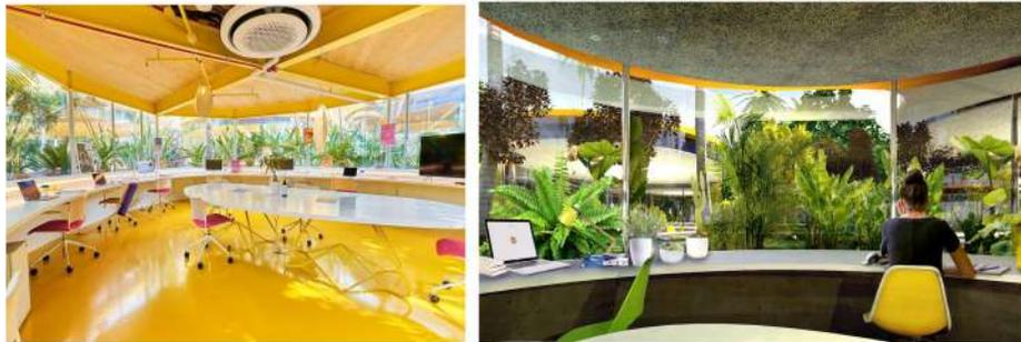
The materials for **the tables and desktops are, a non porous composite material.** Its very durable, seamless materials that allows us to easily build curved shapes. **Walls** - transparent acrylic to provide plenty of natural light and views outside.
