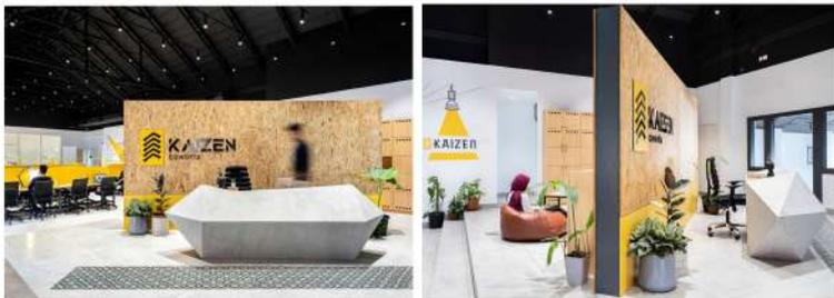
This reception desk is made of **concrete, plywood and metal with storage under**. The reception and the gaming area are separated by an **OSB board partition**.
